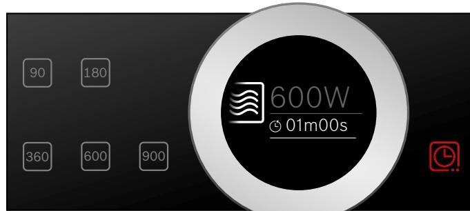
The microwave output and a default cooking time are shown in the display. The ② field lights up red.
