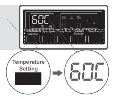
You can gradually decrease the washing water temperature between the maximum temperature and cold washing (--) by pressing washing water temperature adjustment button.
