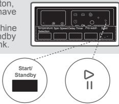
To avoid programme flow from being affected if programme buttons are pressed or programme button is turned when performing washing operation in your machine, child lock is available.
