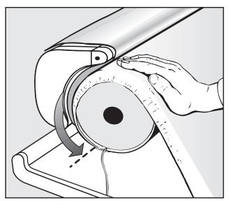
Turn the roller by hand in the direction you iron (see arrow) until the cover retaining slot is at the bottom. Switch on the ironer.
